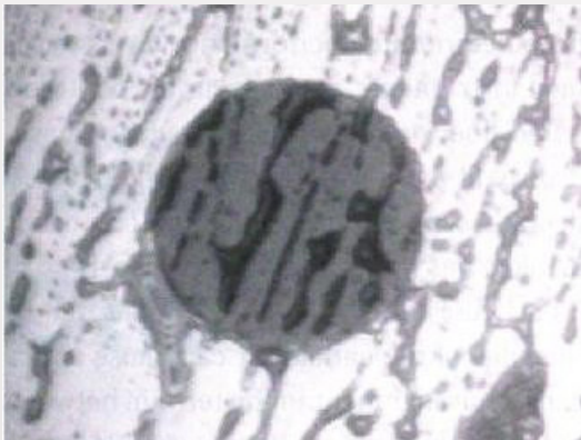
A fiber optic end-face contaminated with fingerprint oil.
