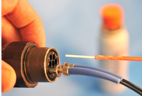
The MIL 38999 connectors require special tools and methods for effective cleaning.
