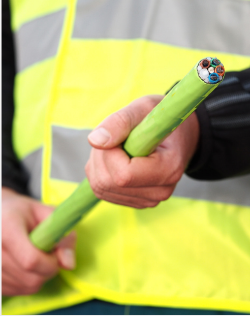
576 fiber cables, like the one here, was once considered large. Many now top out at almost 7,000 strands.
