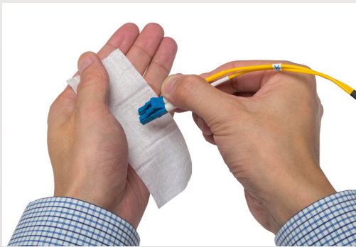
Dry wiping causes static build-up.
