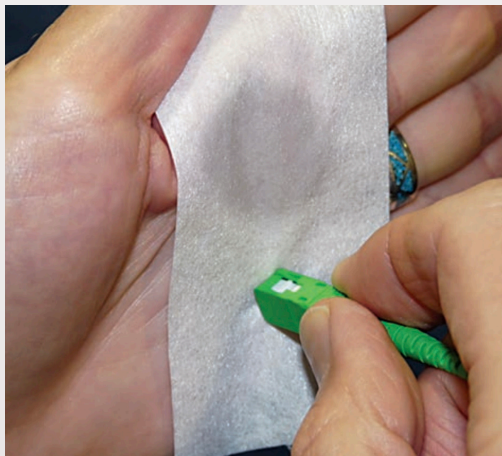
In the old days, many connectors were cleaned by the operator, who just rubbed the connector on his or her shirt or sleeve. That sort of “ad hoc” cleaning will no longer suffice in the world of gigabyte speeds. Operators need the right wipes and the right fluid to get the expected results.
