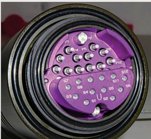
TFOCA connectors are some of the most complex devices on the market. They have ports and jumpers on the same device, which makes cleaning extremely challenging.
