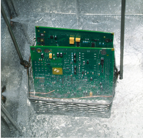
Cleaning fluid cleans tight spaces and under low mounted electrical components
