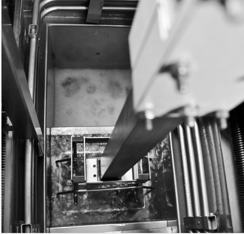
The vapor degreasing machine contains two chambers: the boil sump and the rinse sump.
