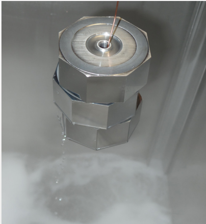
Dirty parts are immersed in cleaning fluid.
