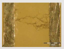
Figure 1: Dendrite growth between two leads
