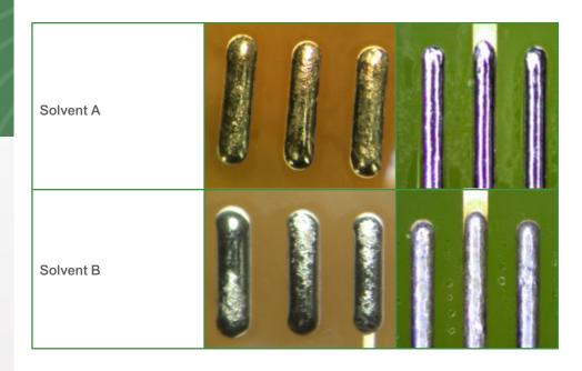
Solvent A was able to clean 7 out of 10 fluxes to 100% flux removal and Solvent B was able to clean 6 out of 10 fluxes to 100% flux removal. The lead-free, no-clean formulations were the most difficult to clean, though all formulations had at least 50% of the flux removed during the cleaning cycle.
