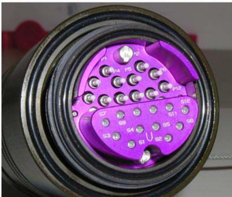
[ Photo, left. A complex military-style high-endurance connector for 24 fibers produced by Fiber Systems International. Notice the "hermaphroditic" nature of the connector -- twelve male connectors and twelve female connectors. This adds strength to the junction. ]
