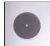
Above: Fingerprint oils on a connector end-face. Right: A properly cleaned connector end-face
