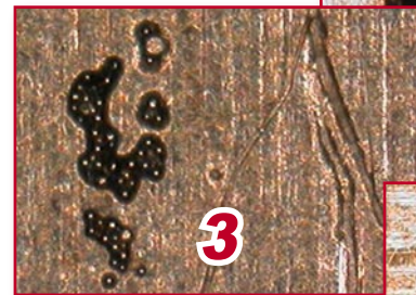
Photos 2, 3 and 4 show the same stencil after 20 printing cycles, wiping without IPA. Easily visible are clogged apertures, fibers from the paper, and excess paste on the stencil, all of which can cause defects in the finished boards
