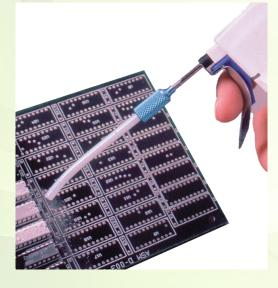
Handy dispensing tool designed to dissipate the ESD charge created by aerosol products. The StatZAP<sup>™</sup> continuously drains static charges to less than 50 volts so the static can never reach levels dangerous to components and PCBs. The StatZAP<sup>™</sup> does not affect or impair solvent performance.
