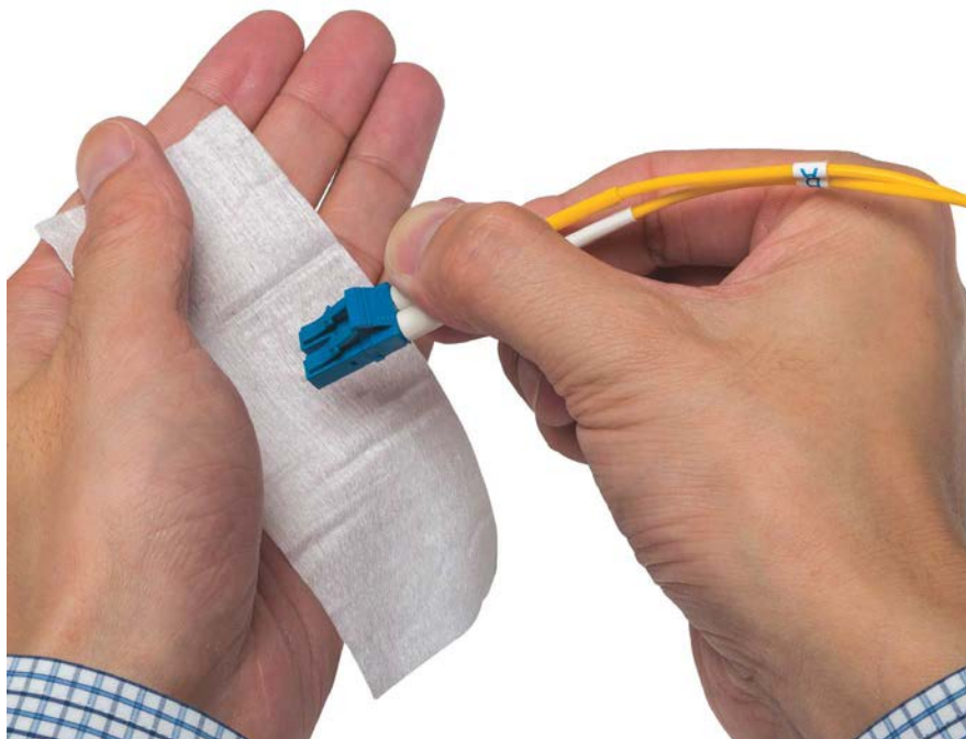
Use fabric wipes to “wet-dry” clean end faces to prevent leaving lint behind.
