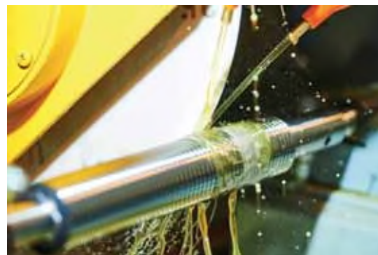
Thread polishing: production debris like machining, stamping or cooling oils, dust, metal filings, marking inks, fingerprints and other soils must be removed
