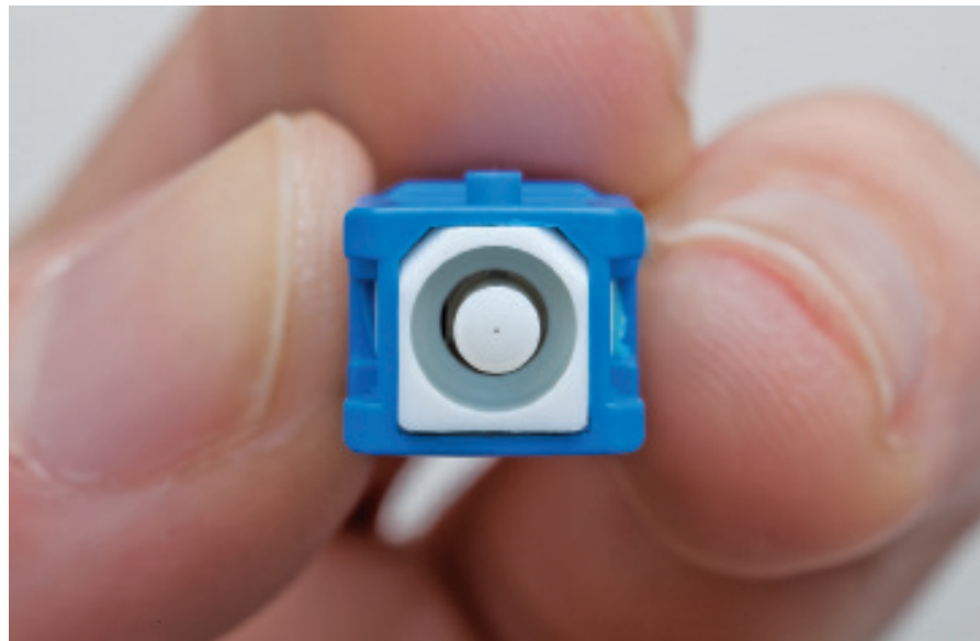
Even brand new, out-of-the-box fiber patch cords must be cleaned. Shown here is an SC connector at the end of such a cord. One of the potentially biggest culprits in new-patch-cord contamination is the dust cap.
