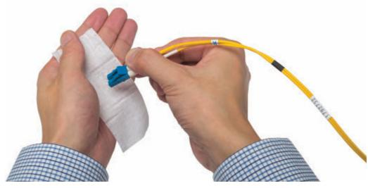
Dry wiping creates a triboelectric charge that attracts unwanted airborne dust to the connector face.
