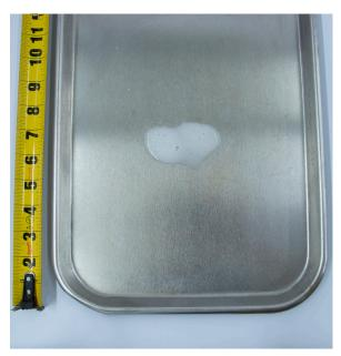
Fig. 3. Actual Spray Coverages of ProEZ Gel™ (Left) and PRE-Klenz (Right), Six-Inch Spray Height
