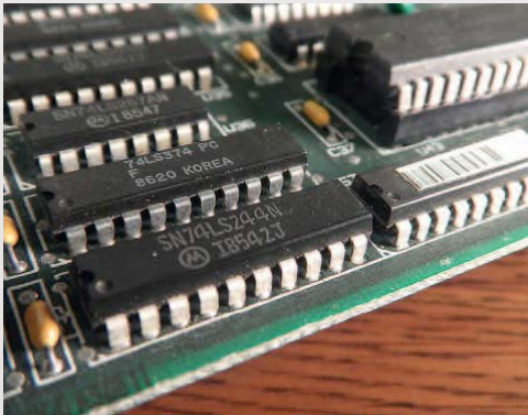
The first through-hole components made their introductions in the commercial applications in the late 1960s - the integrated circuits were embedded in the black plastic housings of the “chips” and the circuits were connected with the long metal legs of the chips, which commonly have 16 to 20 legs.
