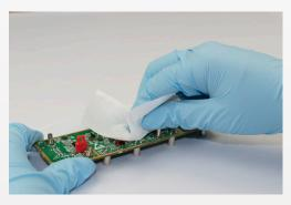
Gently pushing a wipe under low-surface mounted components, quickly dries the PCB.
