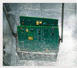
PCBs are cleaned and dried inside a vapor degreaser.
