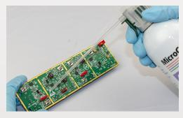
A quick blast from a duster can be effective at blowing trapped moisture from underneath larger components.
