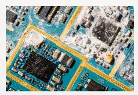
Solder paste and flux needs to be removed for optimal performance.
