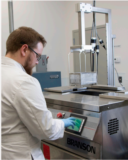
Vapor degreasers offer a simple process that is effective at removing contaminants.
