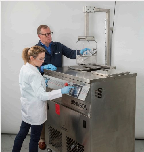
Solvent extraction of up to 80 percent of the binder is done in a vapor degreaser.
