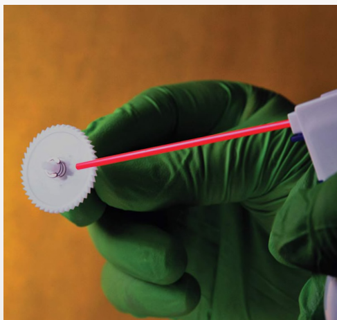
Dry lubricant is often applied to parts using a spray.
