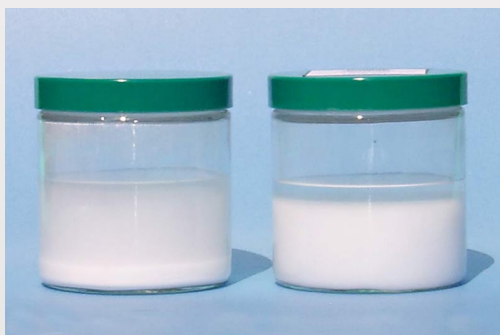
The fluid on the left has a short PTFE “hang time” compared to the MicroCare™ Duraglide™ lubricant on the right.
