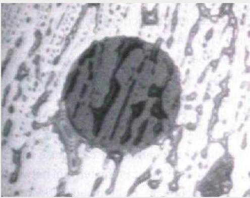
A fiber optic end-face contaminated with fingerprint oil.
