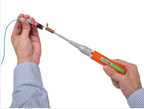
Tools that have a long “throw” pull enough tape or ribbon over the end-face and aren’t contaminated by a soiled alignment sleeve.
