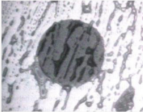
Fingerprint oils contain salts that can create air gaps between the end-faces.
