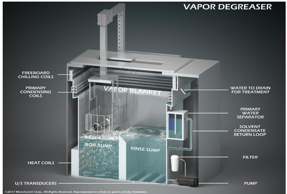
The inner workings of a vapor degreaser are simple, making them cost-effective.
