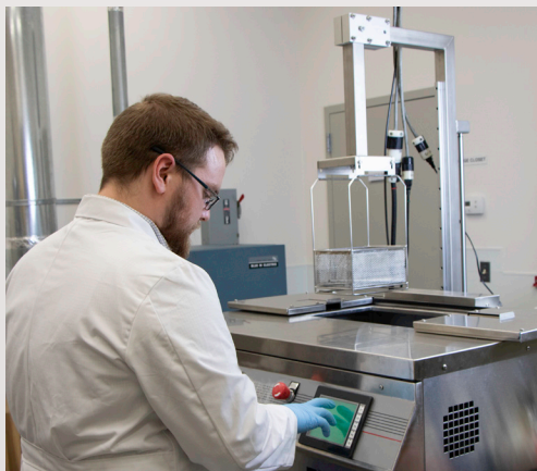
Vapor degreasing using modern fluids is a safe alternative for cleaning.
