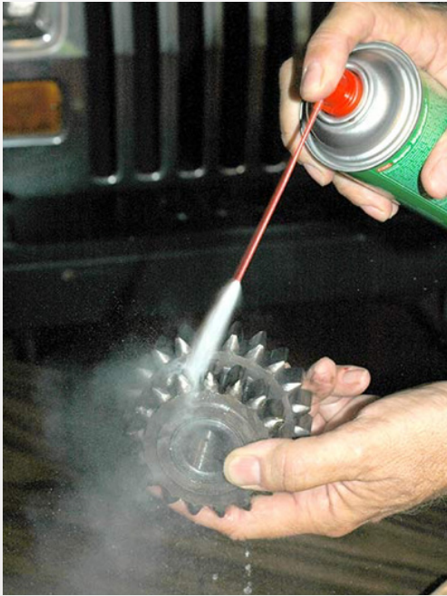
As a solvent, nPB is a powerful degreaser that removes oil and grime quickly. Notice the over-spray from the high-pressure aerosol; this increases worker exposures.
