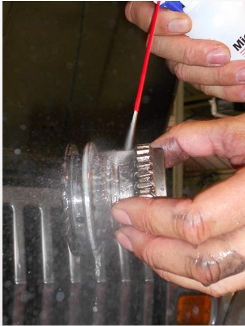
Here the operator cleans a similar gear to excellent results using an HFC-based formulation with a much safer toxicity rating.
