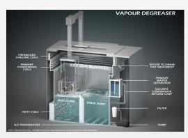
Primary removal of backbone binders can be done with a debinding fluid inside a vapor degreasing machine.
