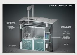
Vapor degreasing uses solvent immersion, combined with vapor rinsing and drying to remove all types of contaminant.
