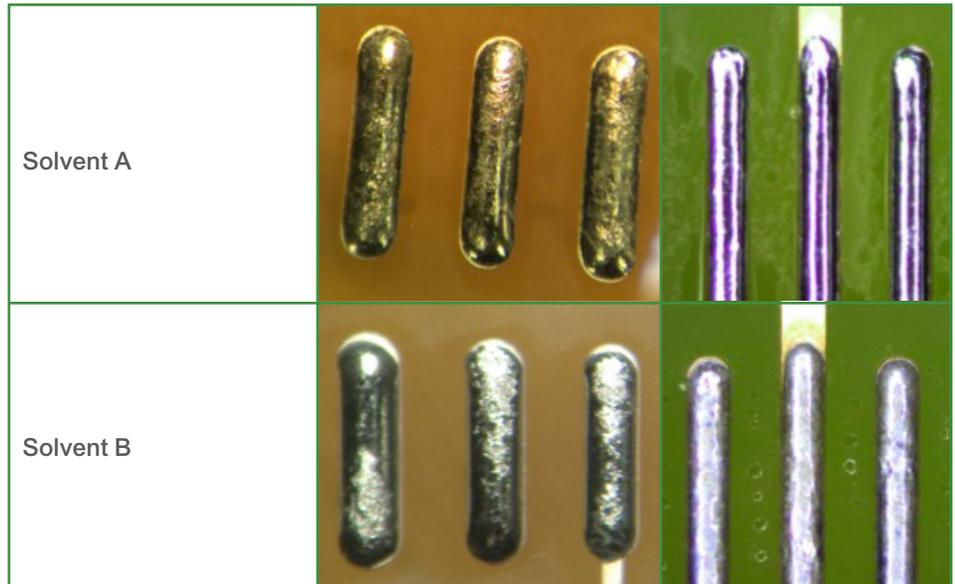
Solvent A was able to clean 7 out of 10 fluxes to 100% flux removal and Solvent B was able to clean 6 out of 10 fluxes to 100% flux removal. The lead-free, no-clean formulations were the most difficult to clean, though all formulations had at least 50% of the flux removed during the cleaning cycle.
