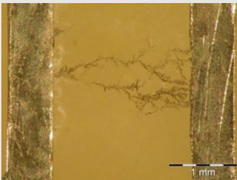
Figure 1: Dendrite growth between two leads
