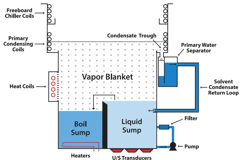
Figure 3: Modern two-sump vapor degreaser.
