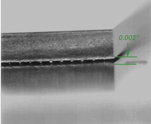
Figure 2: Integrated circuit on a substrate
