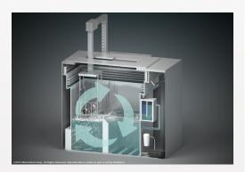
A vapor degreaser recycles cleaning fluid for hundreds of uses, saving waste.
