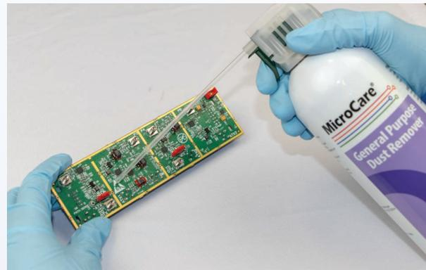
These high-pressure compressed dusters are widely used to remove dry dust and lint from PCBs, optics, machinery, circuitry and keyboards.
