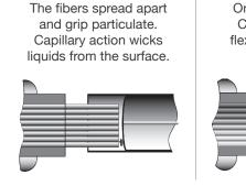
On the head of each CleanStixx<sup>™</sup>, fibers flex to easily conform to the end-face.
