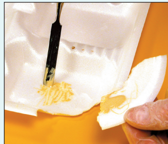
Tear off a portion of the tray wall and use as a small mixing pad.
