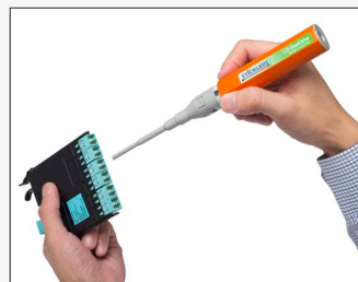
Step 2: Clean the connector end-faces to remove the contamination
