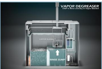
Remove the rinsed parts from the rinse sump and hold in the vapor blanket to drip and dry.
