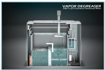
Immerse the cleaned parts into the rinse sump and rinse for 2-10 minutes.
