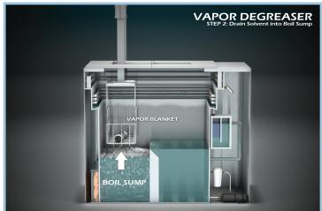
After 2-5 minutes, raise the cleaned parts out of the boil sump and allow them to drain.
