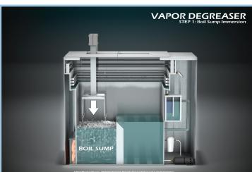
Lower dirty parts through the vapor blanket and into the low-boiling fluid inside the boil sump for cleaning.
