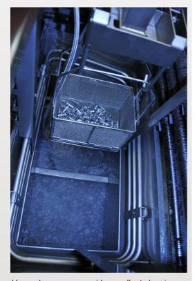
Vapor degreasers provide excellent cleaning results on parts of any size and almost any geometry
