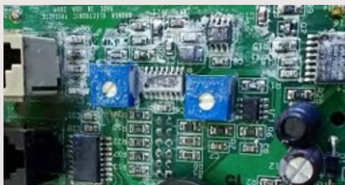
Contaminant includes white residue left behind after soldering the PCB
