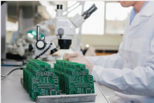
It is essential that the boards are perfectly clean and dry before applying any conformal coatings
