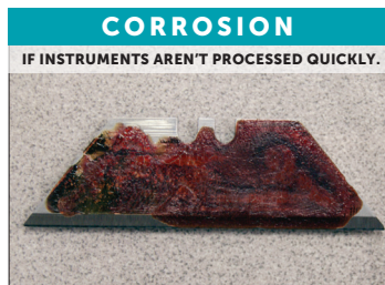
Blades soaked in animal blood surrogate after 15-hour exposure.
