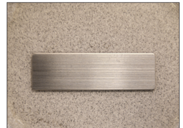
TOSI™ washer test coupon, sprayed with Spec Clean foam and held 72 hours.
