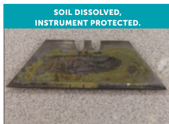
Razor blades after 15-hour soak in Spec Clean foam show corrosion arrested and soils dissolved.
