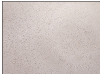
Spec Clean foam is applied to TOSI™ washer test coupon. Foaming properties of product in use.
