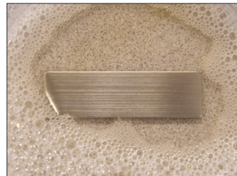
Test results after 15 hours show Spec Clean foam has dissolved soils and remains liquid for easy rinsing.
