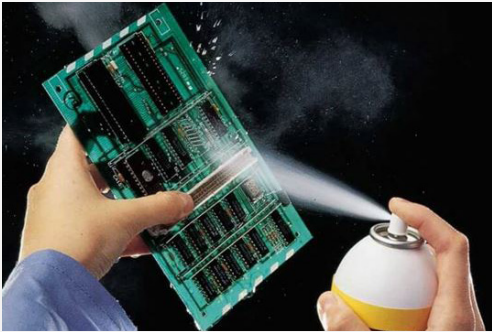
Aerosol cleaning is messy and expensive due to the high volume of wasted cleaning fluid.
