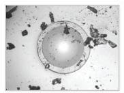
Dust contamination on an end face.
