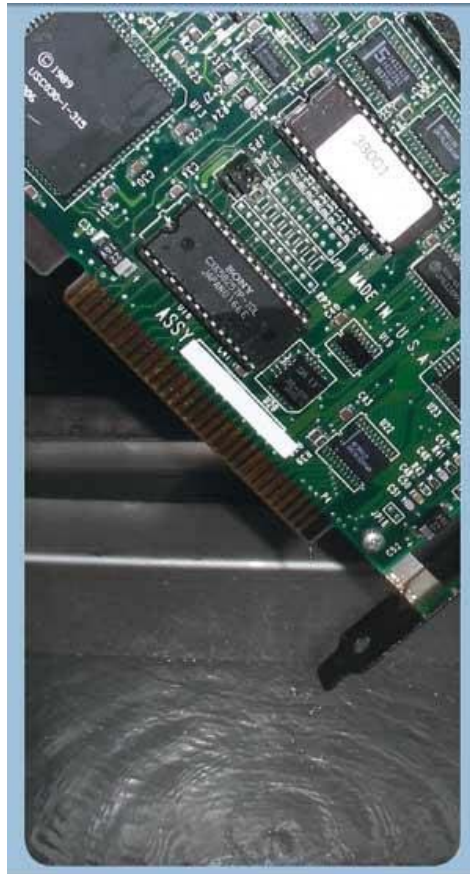
Figure 2. The board, being relatively cold, causes the vapors to condense onto its surface, dissolving contamination and allowing it to drip down into the liquid solvent.
