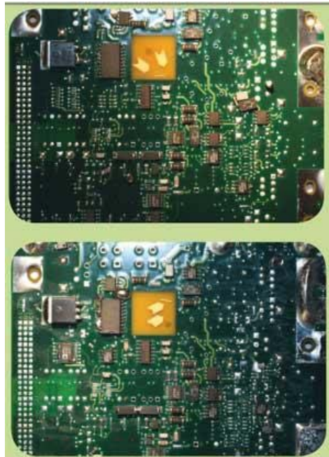
Figures 1A & B. Poor cleaning can result in white residues (B) that detrimentally affect inspection and PCB performance.
